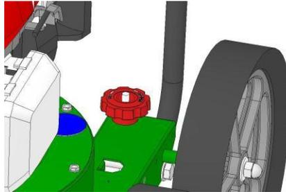
**FOR MAXIMUM PICKUP:** Adjust nozzle close to debris, but without blocking airflow into the nozzle. *NOTE:* Never bury nozzle into debris.
