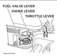
Pull the engine recoil handle slowly until it engages then pull hard and fast to start the engine.
