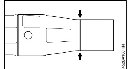
The front end of the nozzle is worn by ground contact during operation. Replace the nozzle when it has worn as far as the wear mark.
